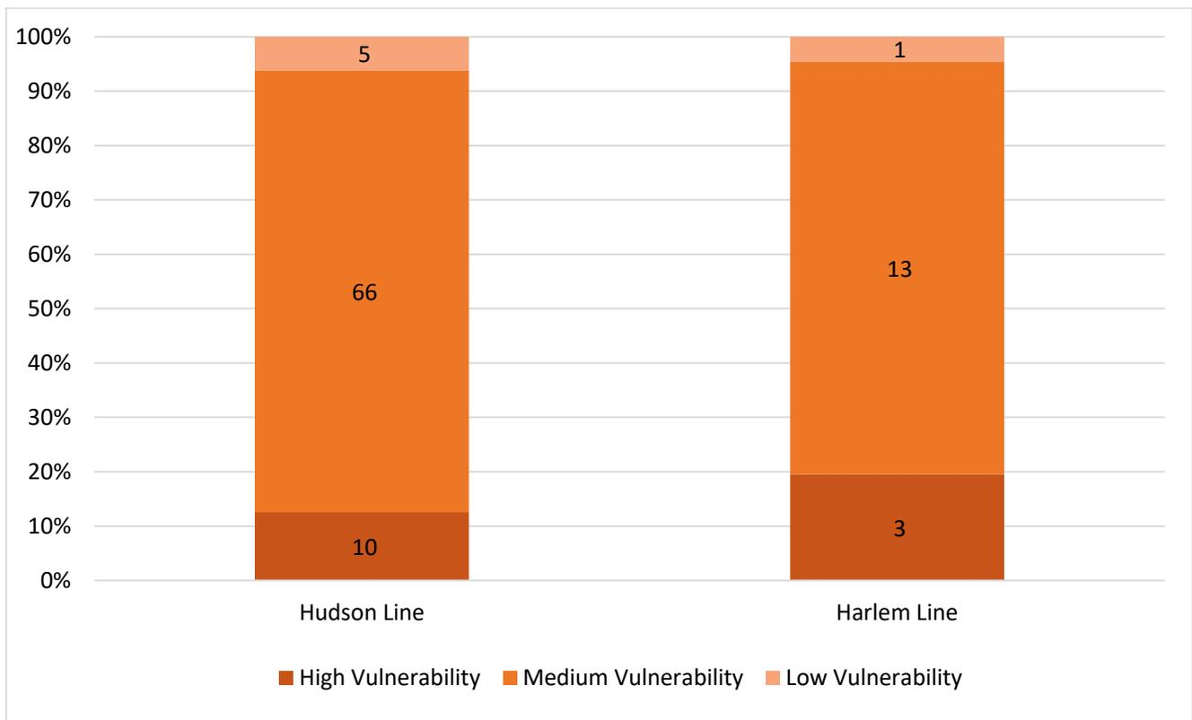
**FIGURE 7. PERCENTAGE AND COUNT OF RAIL LINE MILES WITH HIGH, MEDIUM, AND LOW FLOOD VULNERABILITY**
