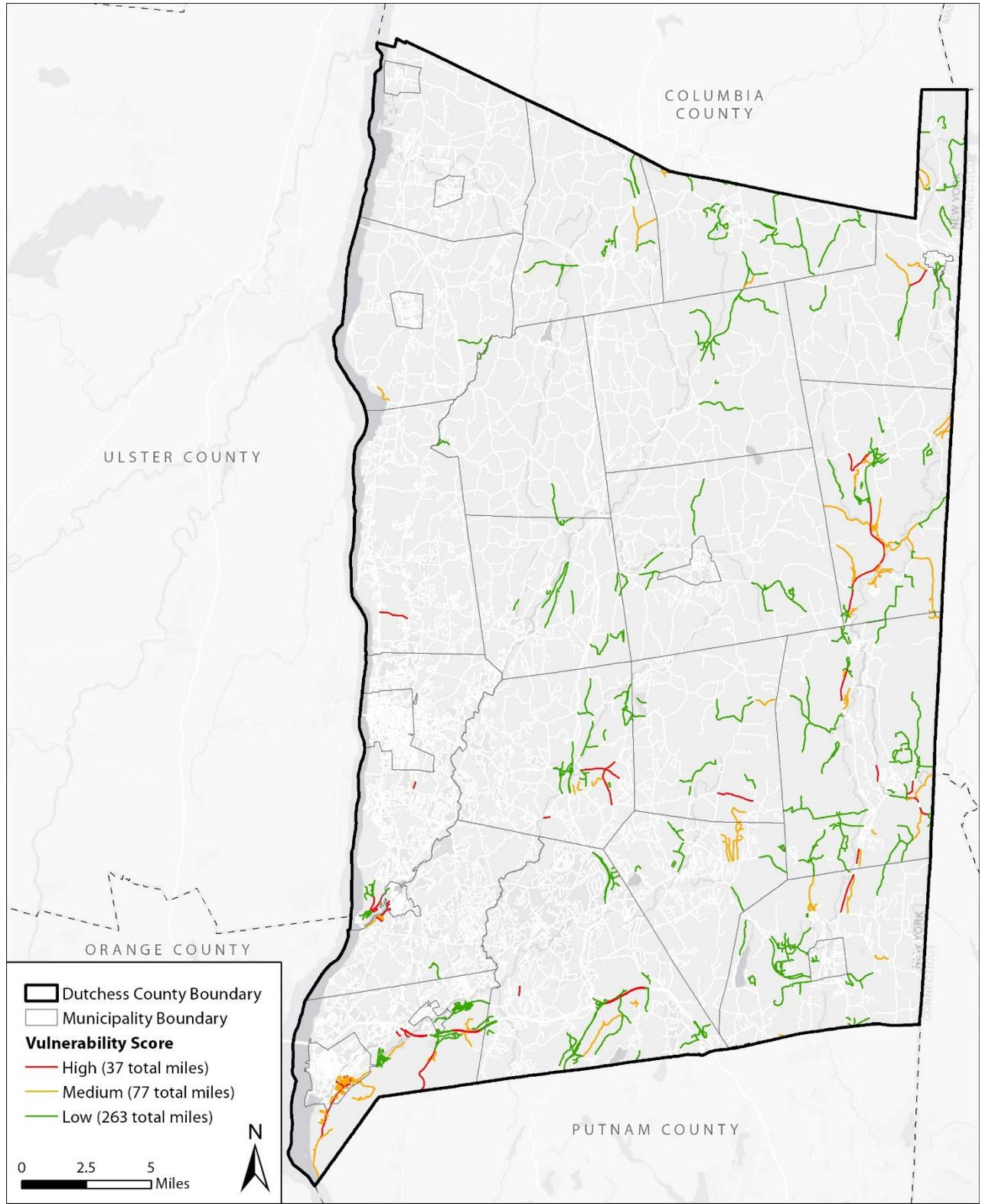
**Landslide Vulnerability for Roads**
